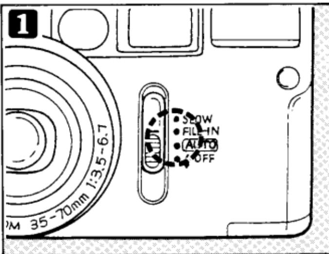
[E] Press the shutter button lightly and confirm that the flash indicator lamp (orange) lights.
